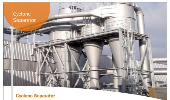
Cyclone dust removal is a preliminary filtration device for air purification system. The cyclone series of Kaisen has rational design, simple structure and adopts axial access type. Treatment of air flow is 3 times that of common cyclone dust removal, and air stream is distributed evenly.
